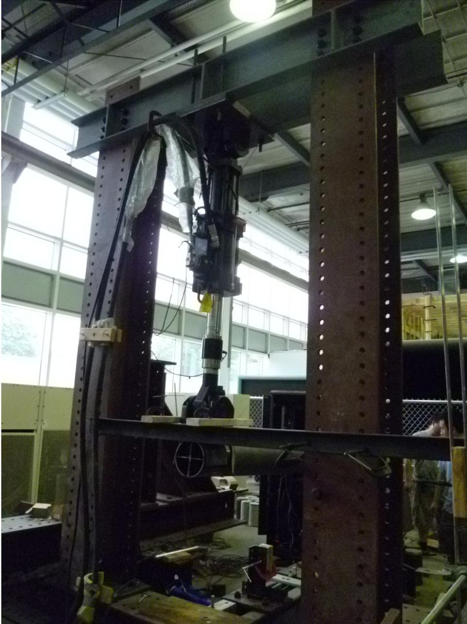
Figure 3. Fatigue test setup for full scale piezo paint sensor characterization test
