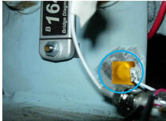
Figure 9. Piezoelectric paint AE sensor (blue circled, for monitoring ambient noise since there is no fatigue crack on this side connection plate)
