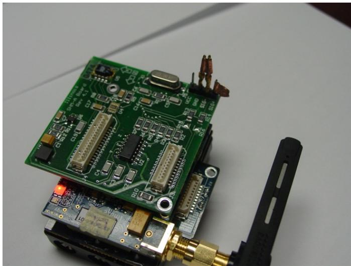
Figure 12. Wireless sensor Imote2 (measuring acceleration and temperature)
