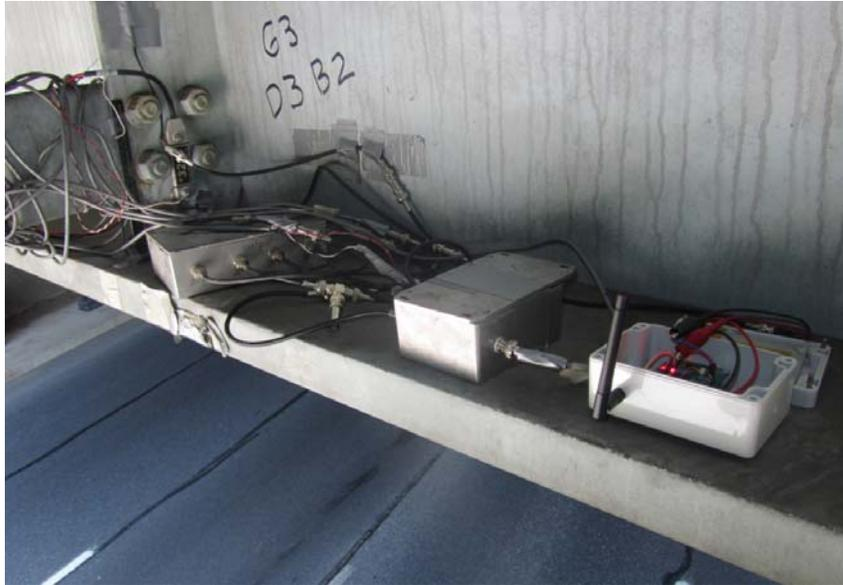
Figure 9. System set up overview with the wireless sensor
